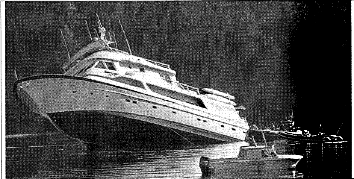
Figure 4. According to crewmembers, the Safari Spirit listed to starboard at an angle of about 35° when it shifted on the submerged rock. Photograph courtesy of Shearwood Marine.
