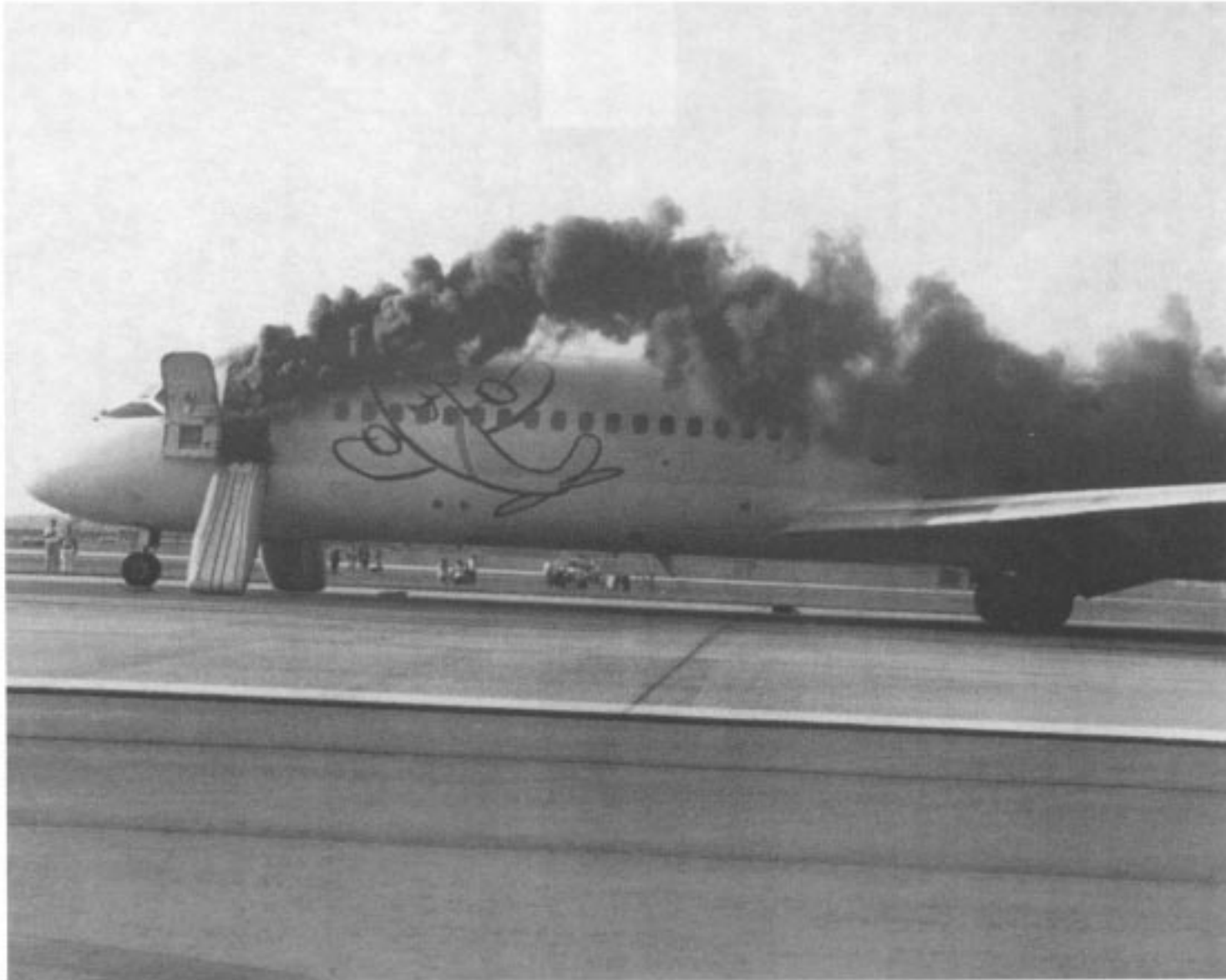
Figure 3—Photograph of flight 597 after uncontained engine failure
