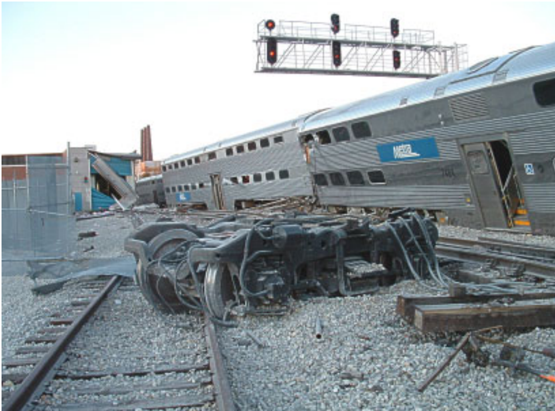
Figure 3. All five passenger cars derailed but remained upright. The trucks from the lead locomotive dislodged (foreground).
