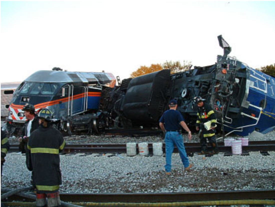
Figure 2. The lead locomotive (on its side) and second locomotive at their final resting positions.
