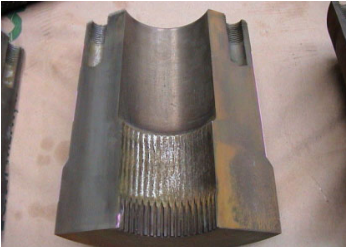
Figure 13. Section of planetary gear receiving hub showing stripped splines.
