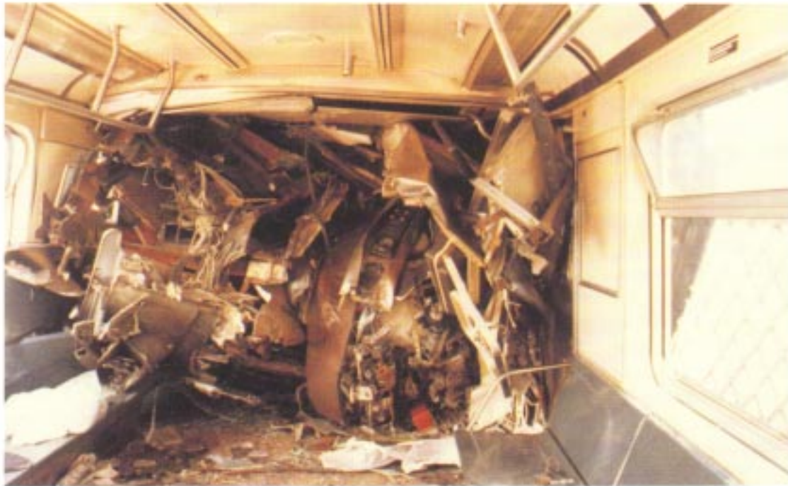
Figure 7 — Interior damage to the lead car of the J train.
