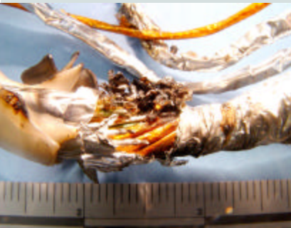
Heat damaged wiring from the Genesis spacecraft.
