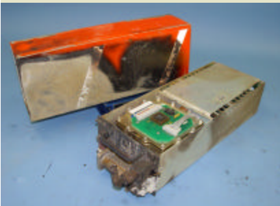
The flight data recorder from the Jetstream 32, which crashed near Kirksville, MO.
