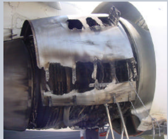
The recent engine fire on a Blue Panorama Boeing 767 in Rome, Italy
