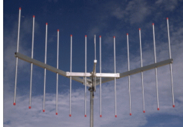
Figure 13. A typical corner-reflector antenna
