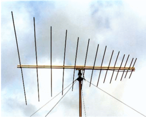
Figure 19. A typical log-periodic antenna
