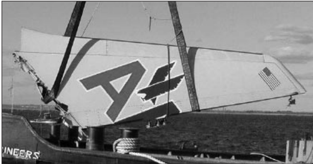
Figure 4. Vertical stabilizer as recovered from Jamaica Bay.
