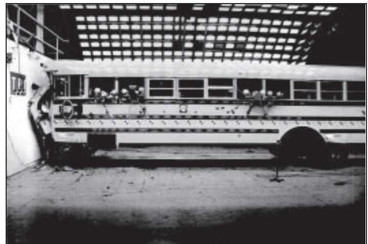
Figure 9. The school bus in the frontal impact scenario after the impact.
