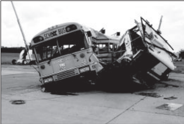
Figure 13. The heavy truck relative to the side of the school bus after impact.
