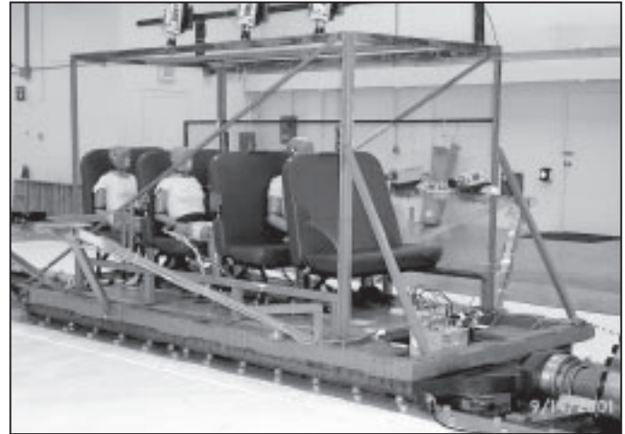
Figure 16. A photograph of the modified sled buck used in the second test series.
