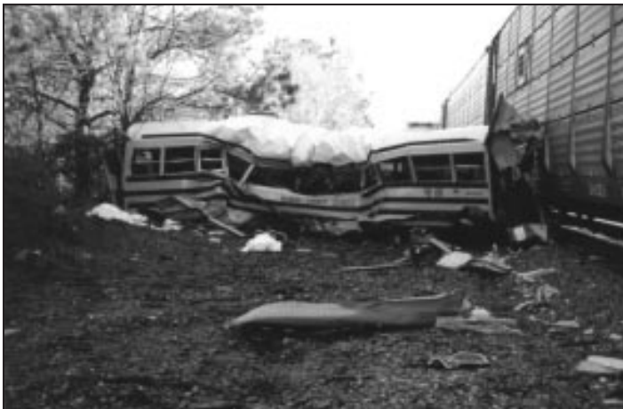
Figure 4. The bus body came to rest against the side of the train (Conasauga, Tennessee).
