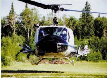
Bottom left: Wallops Flight Facility's Bell Huey helicopter, carrying two side platforms with a POLDER instrument, a modular multi-band radiometer (MMR), an SE-90 spectrometer, infrared thermal (IRT) sensors, and video recording equipment. Pictured here, the helicopter is participating in the BOREAS campaign, near Prince Albert, Saskatchewan, Canada (NASA Ames Research Center).
