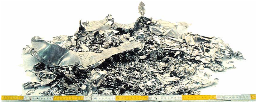
Figure VI-3. RMI Debris Observed in Siemens Steam-Jet Impact Tests
