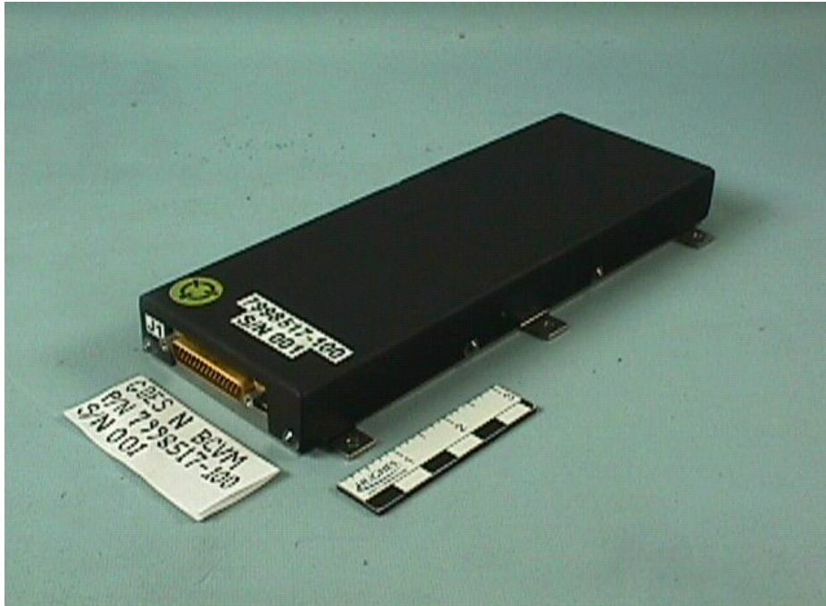
Figure 10-6. Battery Cell Voltage Monitor
