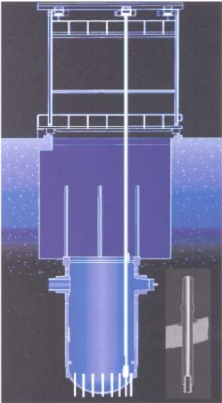
The scanning manipulator is positioned on the nozzle with a rigid pole system.
