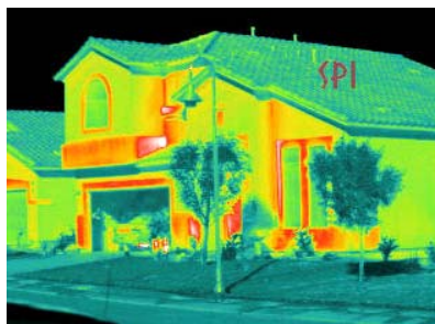
Residential Thermal Energy Loss
