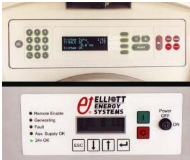
Front control panels of Capstone and Elliott microturbines
