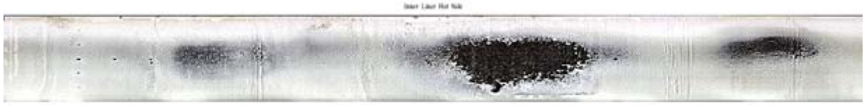
Figure 1. Gas-path surface of inner liner from Chevron engine test #6 showing localized loss of Si/BSAS EBC.
