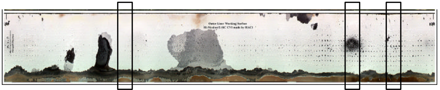
Figure 2. A series of compiled images showing the entire working surface of the outer liner after 13,937 h engine test.
