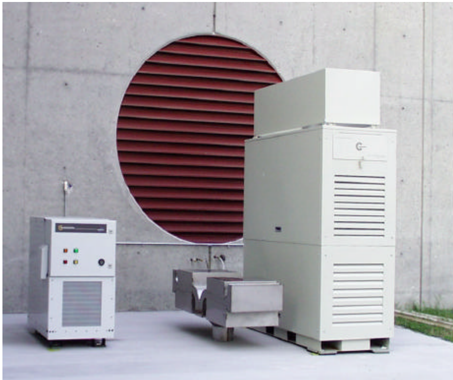
Figure 1. Microturbine test facility. On the left is a 100 psi gas compressor. On the right is the modified 60kW Capstone microturbine. Next to the microturbine is an exhaust noise suppressor.
