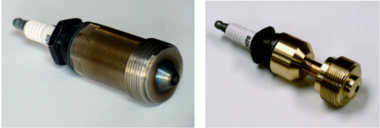
Fig. 1 Original (left) and modified (right) rotating arc spark plugs.
