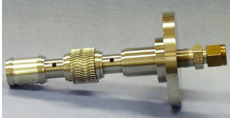
Figure 2. Photograph of sample holder for evaluation of foil test specimens. Note plain and corrugated foil test specimens at locations 1 and 3 of the sample holder.
