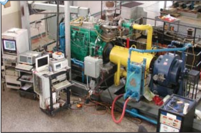
Cummins, in conjunction with Colorado State University, is testing diesel pilot injection on a QSK19G gas engine.
