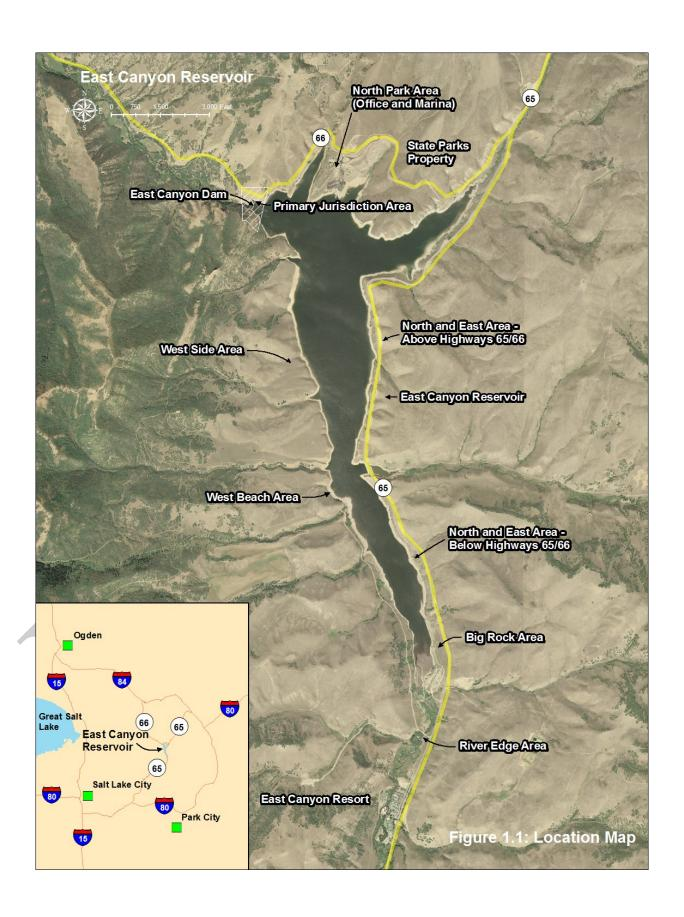
Water released from East Canyon Dam is returned back to East Canyon Creek, where it flows to the Weber River and is diverted for domestic and irrigation uses. The present dam nearly doubled the East Canyon Reservoir water storage capacity from 28,800 acre-feet to 51,200 acre-feet. The DWCCC, through an agreement with Reclamation and the Weber Basin Water Conservancy District, operates and maintains East Canyon Dam.
