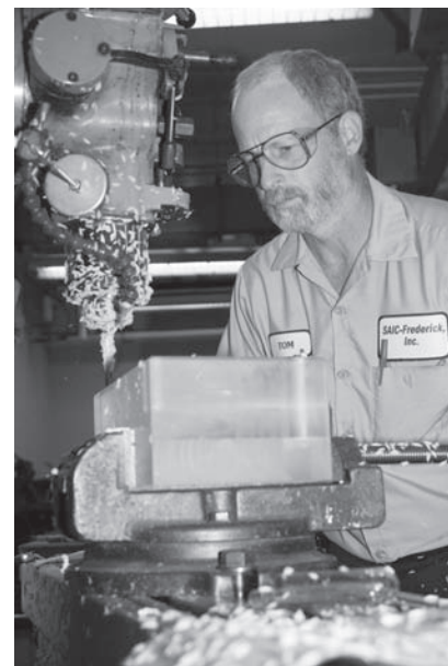
FME machinist Tom Crone mills an acrylic block to create a test tube holder.
