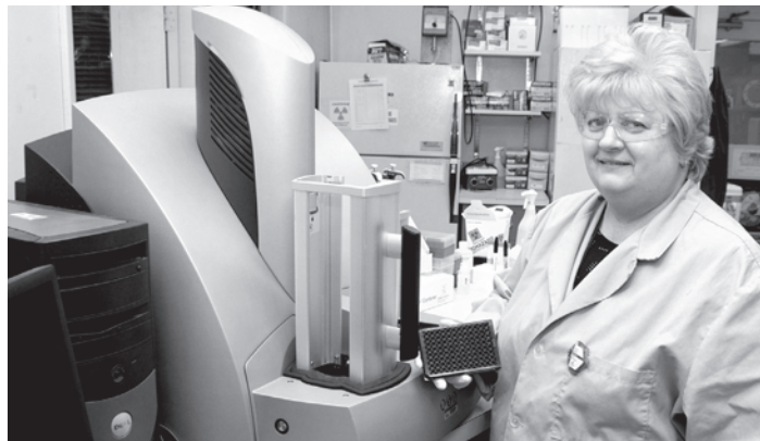
Helen Rager, Associate Scientist at the Clinical Support Laboratory, Applied/Developmental Directorate, holds a test plate from the Meso Scale Discovery SECTOR Imager 6000, used for high-throughput multiplex assays for cytokines, growth factors, and phosphoproteins.
