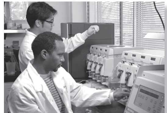
Garrison Owens (foreground) and Dr. Chang Hee Kim, LMT scientists, work at an Affymetrix high-density microarray work station, an instrument used for cancer gene discovery and detection studies.
