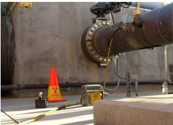
No. 2- Radiography test equipment. Metal box at center is housing for source which is deployed using yellow cable. Film and tape with lead reference numbers are at photo right, Geiger counter at left.
