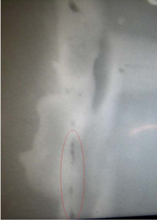
No. 5- Portion of radiograph of weld at CH-33B L1. Dark spots in a line (circled) indicate lack of fusion.
