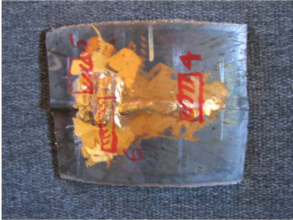
Figure 2. Pipe sample marked for metallurgical sample removal.
