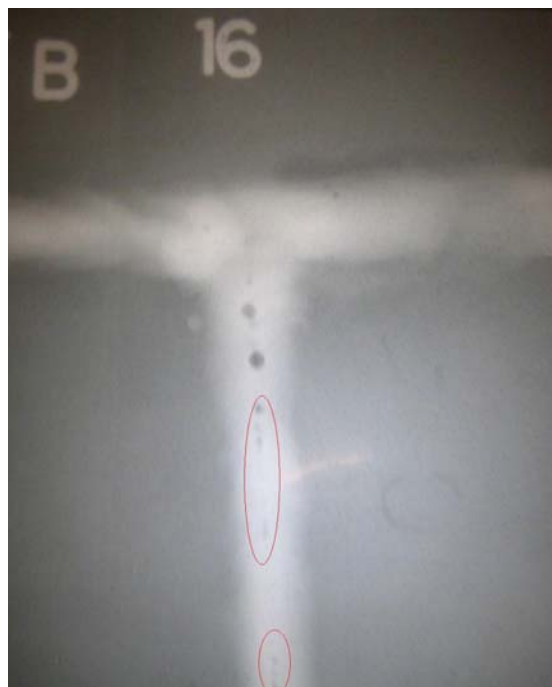
No. 4- Portion of radiograph of weld at CH-9 C1. Dark spots in a line (circled) indicate incomplete penetration.
