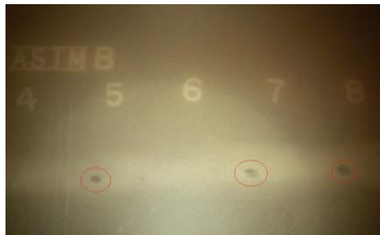
No. 3- Portion of radiograph of weld at CH-10 L1. Dark spots (circled) show porosity.
