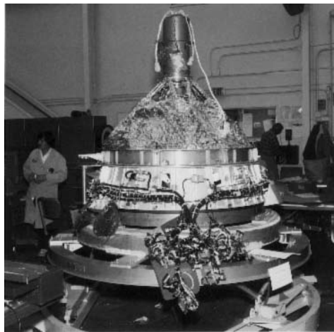
Figure 5.2. Galileo’s despun section receives its cabling.
