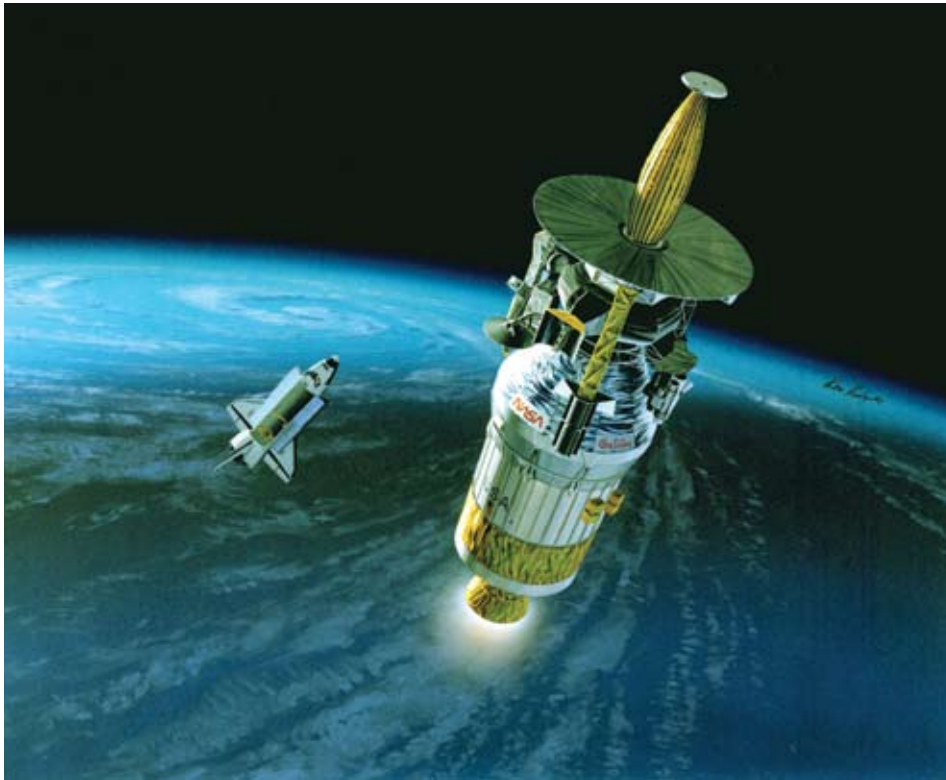
Figure 6.1. The deployed Galileo spacecraft and Inertial Upper Stage booster rocket. Note the two circular sun shields installed to protect the spacecraft's sensitive equipment. (Image number S89-42940)
