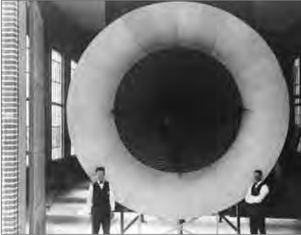
Two wind tunnel researchers pose near the entrance end of Langley's five-foot Atmospheric Wind Tunnel (AWT), where air was pulled into the test section through a honeycomb arrangement meant to smoothen the flow. NASA Image #L-1990-04342 (LaRC)
