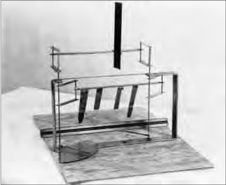
Reproduction of the 1901 Wright drag balance. Orville actually built two balances, one for lift measurements and the other for drag. Model airfoils could be mounted on both balances and easily changed. Lift and drag forces calculated from these measurements clearly indicated that the previously accepted aerodynamic coefficients on which the design of airfoils were being based were grossly in error. SI Negative No. A-41899-B
