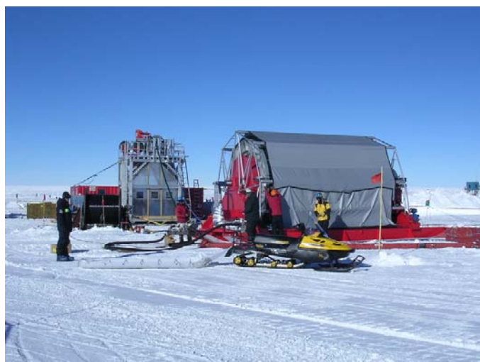
January 9, 2005: Tower, drill cable connected, hose end in tower. Second drill shift installing a windbreaker to reduce heat loss. Credit: the United States Antarctic Program.
