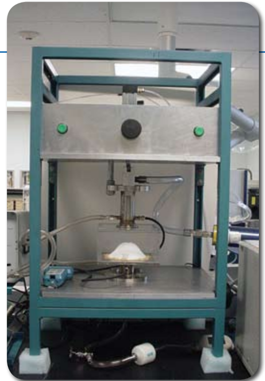
A flat plate test system for measuring respirator filter penetration of 3 to 20 nm silver particles
