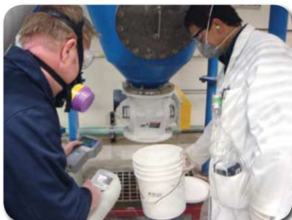
NIOSH monitoring of a worker during a nanomaterial powder production and collection.
