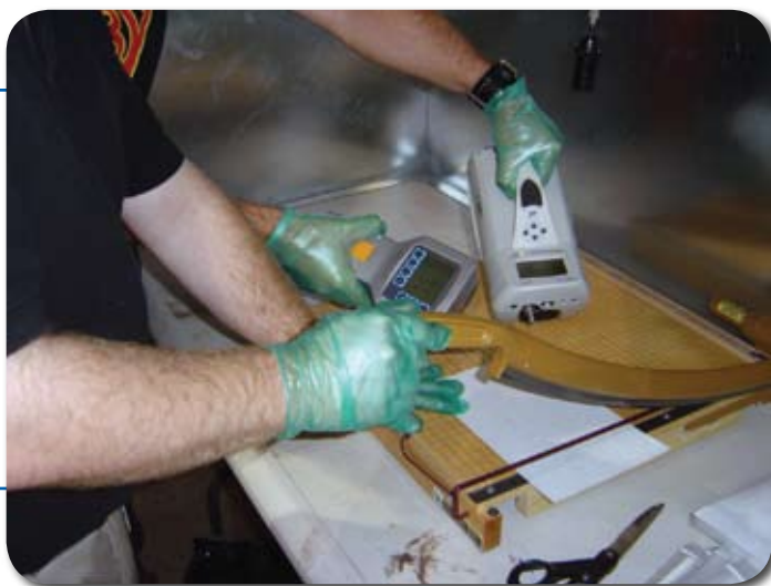
Checking for fiber release during destructive testing of nanofibers deposited on a substrate using optical and condensation particle counters.
