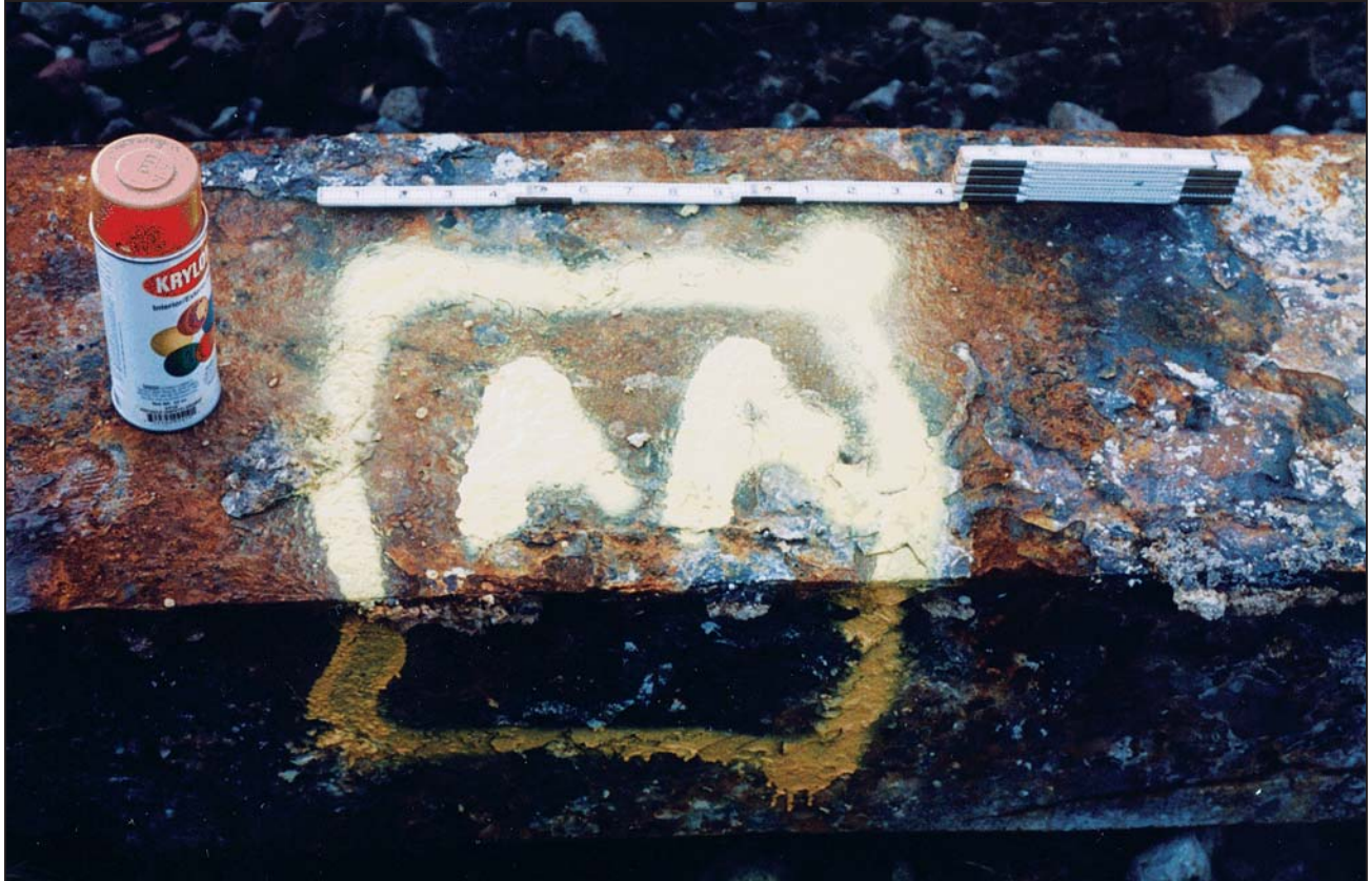
Figure D-11 Burnt steel piece marked for cutting of coupon.
