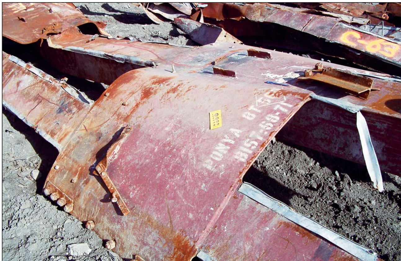
Figure D-5 Stenciled markings on WTC 2 perimeter column from floors 68–71.
