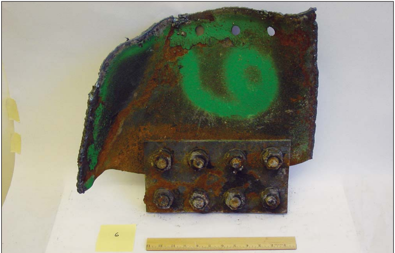
Figure D-12 Coupon cut from WTC 5 showing web tear-out at bolts.
