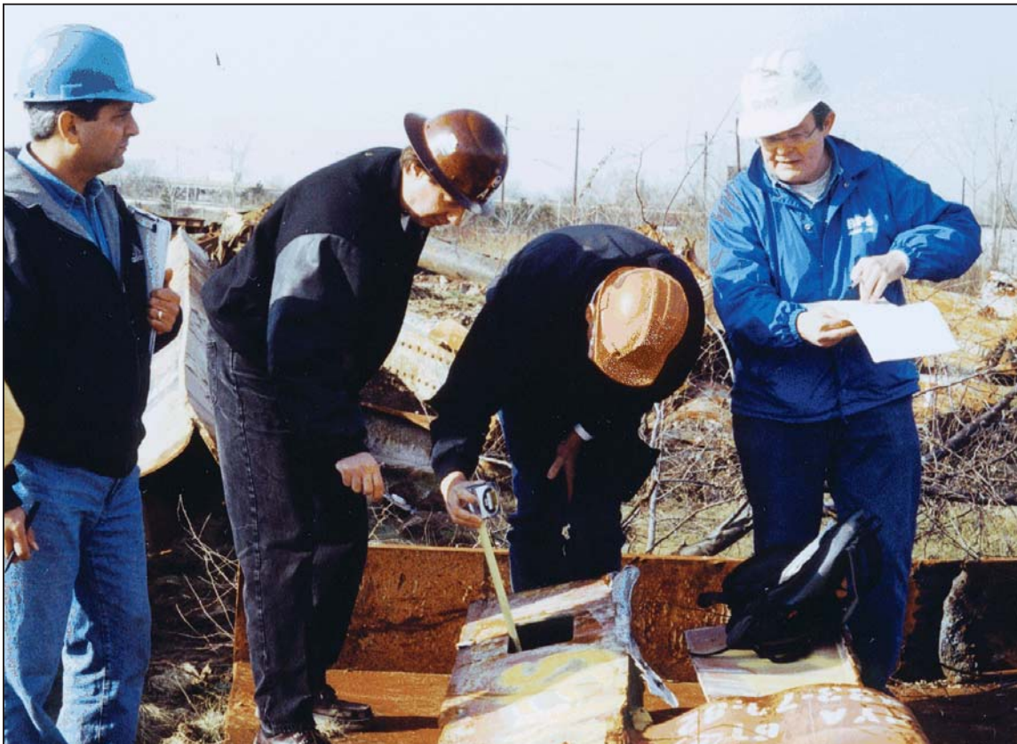
Figure D-7 Engineers measuring and recording steel piece dimensions.
