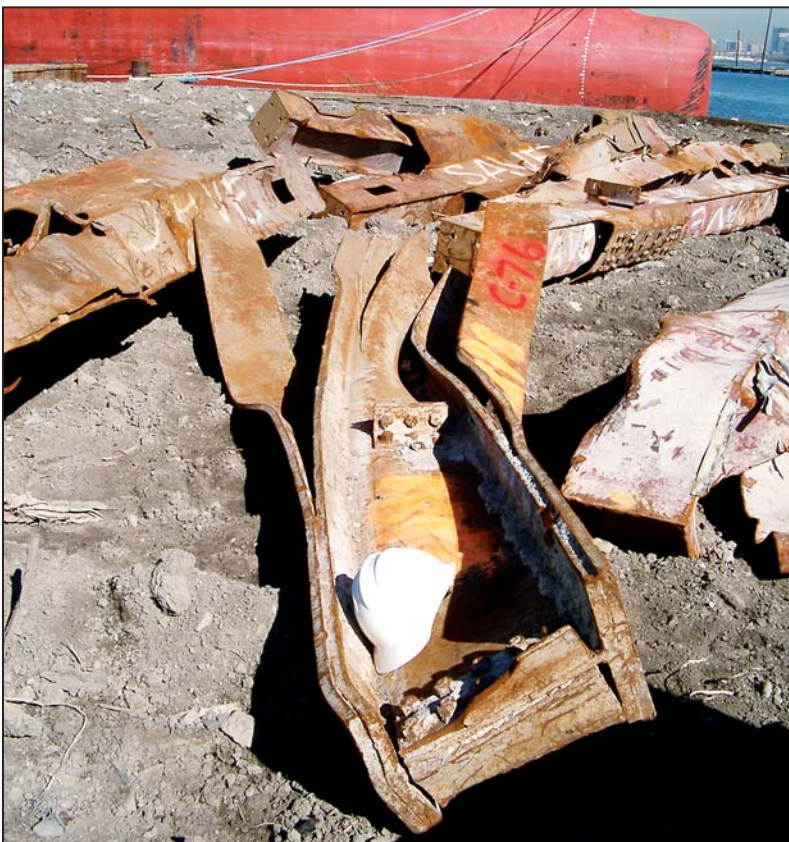
Figure D-14 WTC 7 W14 column tree with beams attached to two floors.
