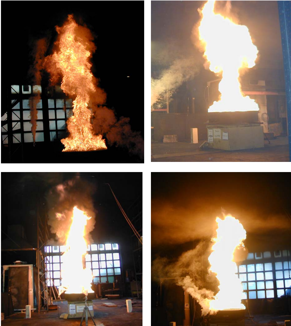
Figure A-22. Photographs of Heptane Pan Fires, ICFMP BE #2, Case 2 (Courtesy, Simo Hostikka, VTT Building and Transport, Espoo, Finland)
