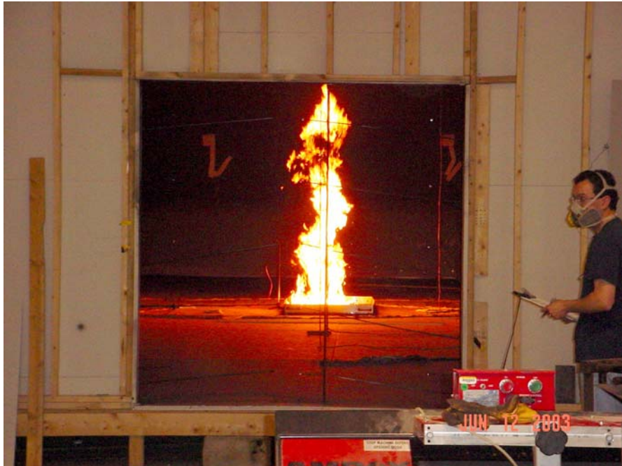
Figure A-19: Photographs of ICFMP BE #3, Test 3, as seen through the 2 m by 2 m Doorway, Courtesy of Francisco Joglar, SAIC
