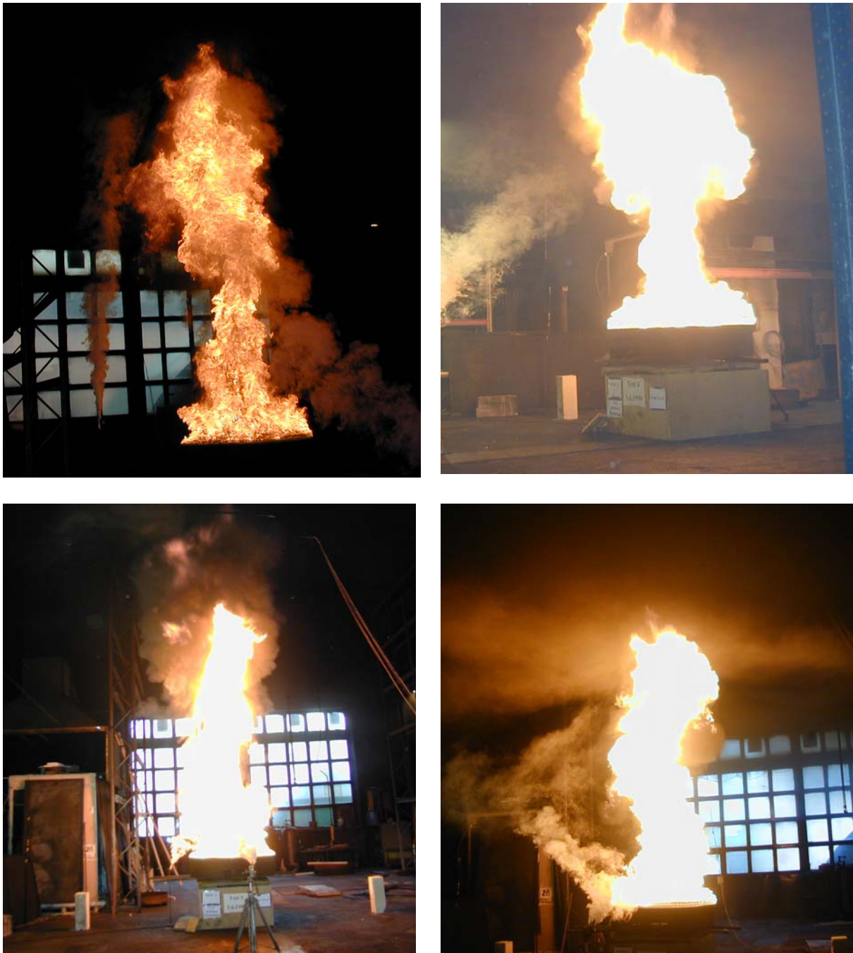
Figure A-18: Photographs of Heptane Pan Fires, ICFMP BE #2, Case 2, Courtesy of Simo Hostikka, VTT Building And Transport, Espoo, Finland
