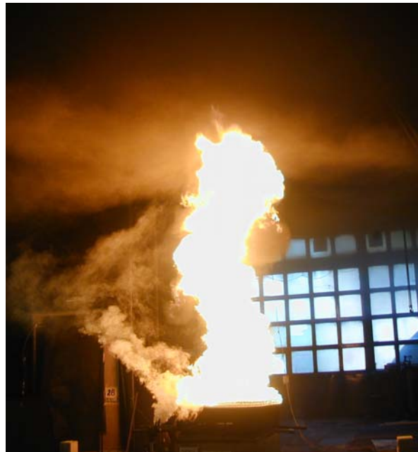
Figure A-12: Photographs of Heptane Pan Fires, ICFMP BE #2, Case 2 (Courtesy of Simo Hostikka, VTT Building and Transport, Espoo, Finland)
