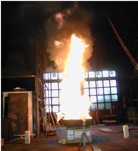
Figure A-12: Photographs of Heptane Pan Fires, ICFMP BE #2, Case 2 (Courtesy of Simo Hostikka, VTT Building and Transport, Espoo, Finland)
