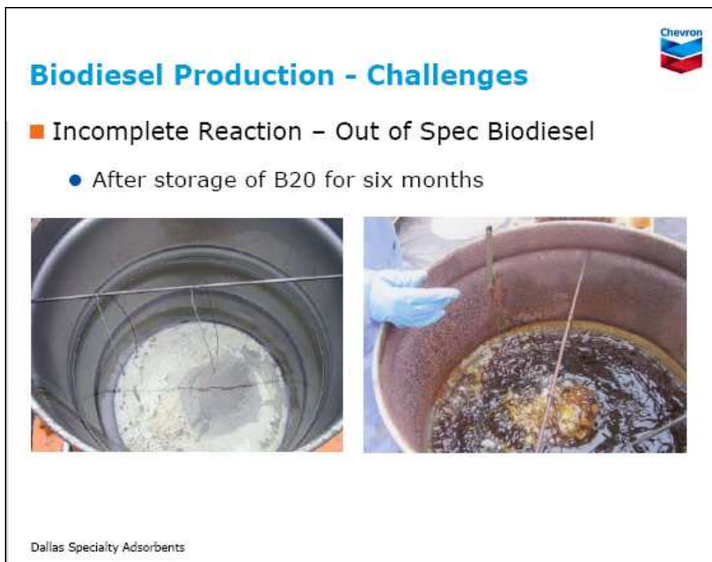
Figure 7. “Poor shelf life” of B20 resulting from production problems that result in excessive amounts of mono-, di-, and tri-glycerides
