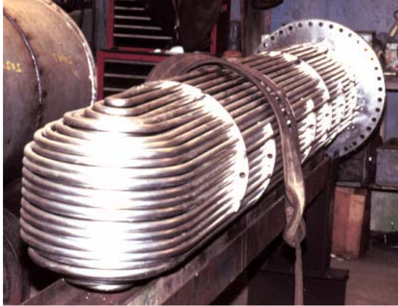
Figure 3.7. Steam Generator U-Tube Bundle
