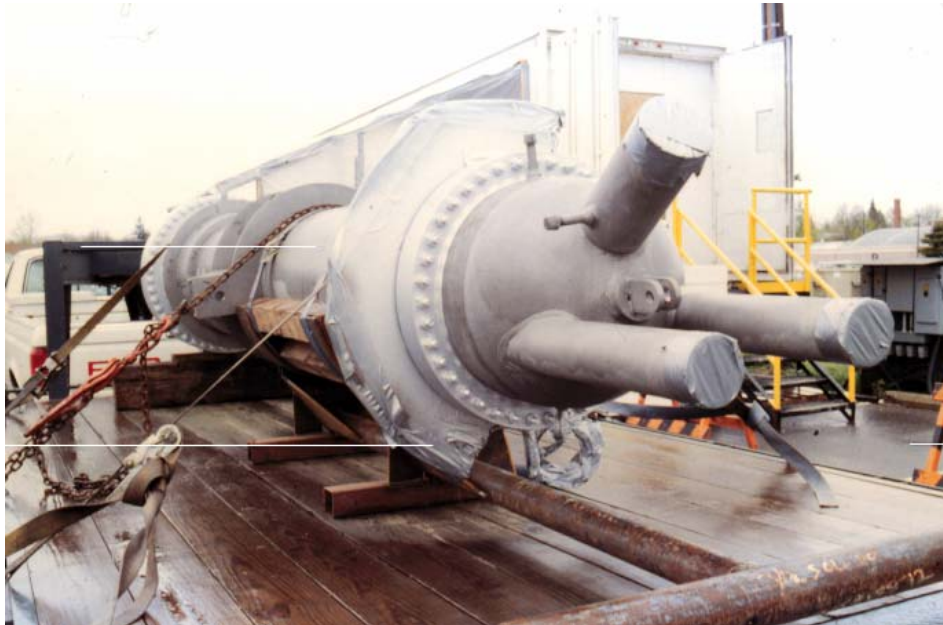
Figure 3.6. Steam Generator Being Delivered to the APEX Facility
