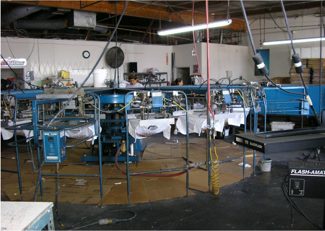
Figure 2-8. Automated Press at Powerhouse
