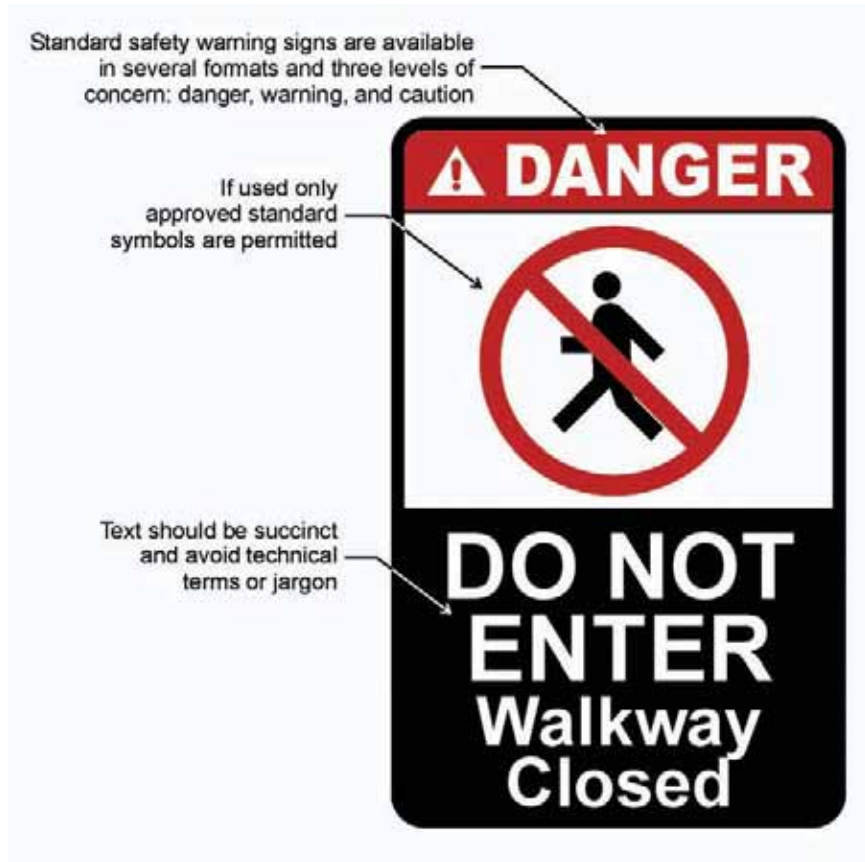
Design Type G – Regulatory/Warning/Security Sign
