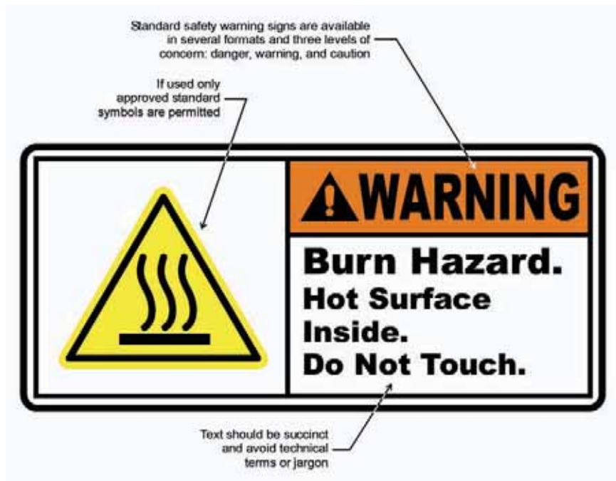
Design Type G – Regulatory/Warning/Security Sign
