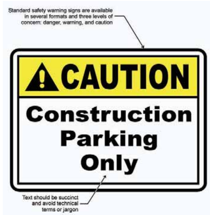
Design Type G – Regulatory/Warning/Security Sign
