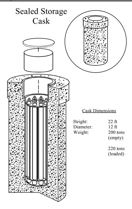
The container would be a large storage cask that would hold the high-level radioactive waste.
