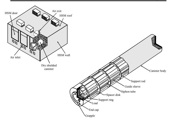
After several years, the heat generated by the decay of the fission products decreases sufficiently to allow the storage of the spent fuel in an air-cooled, dry, above ground storage facility. These facilities must be designed to remove the heat from the spent fuel and be designed to limit the radiation in the areas around the facilities.
