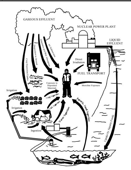
Gaseous and liquid radioactive wastes, after processing, may be released to the environment. This can result in the exposure of members of the public. The diagram above shows some of the pathways that could result in the exposure of a member of the public.
