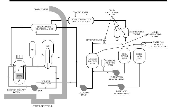
The chemical and volume control system (CVCS) on a pressurized water reactor is used to remove the activation products and fission products from the reactor coolant. It will be used to show some of the sources of solid, liquid, and gaseous radioactive wastes.
