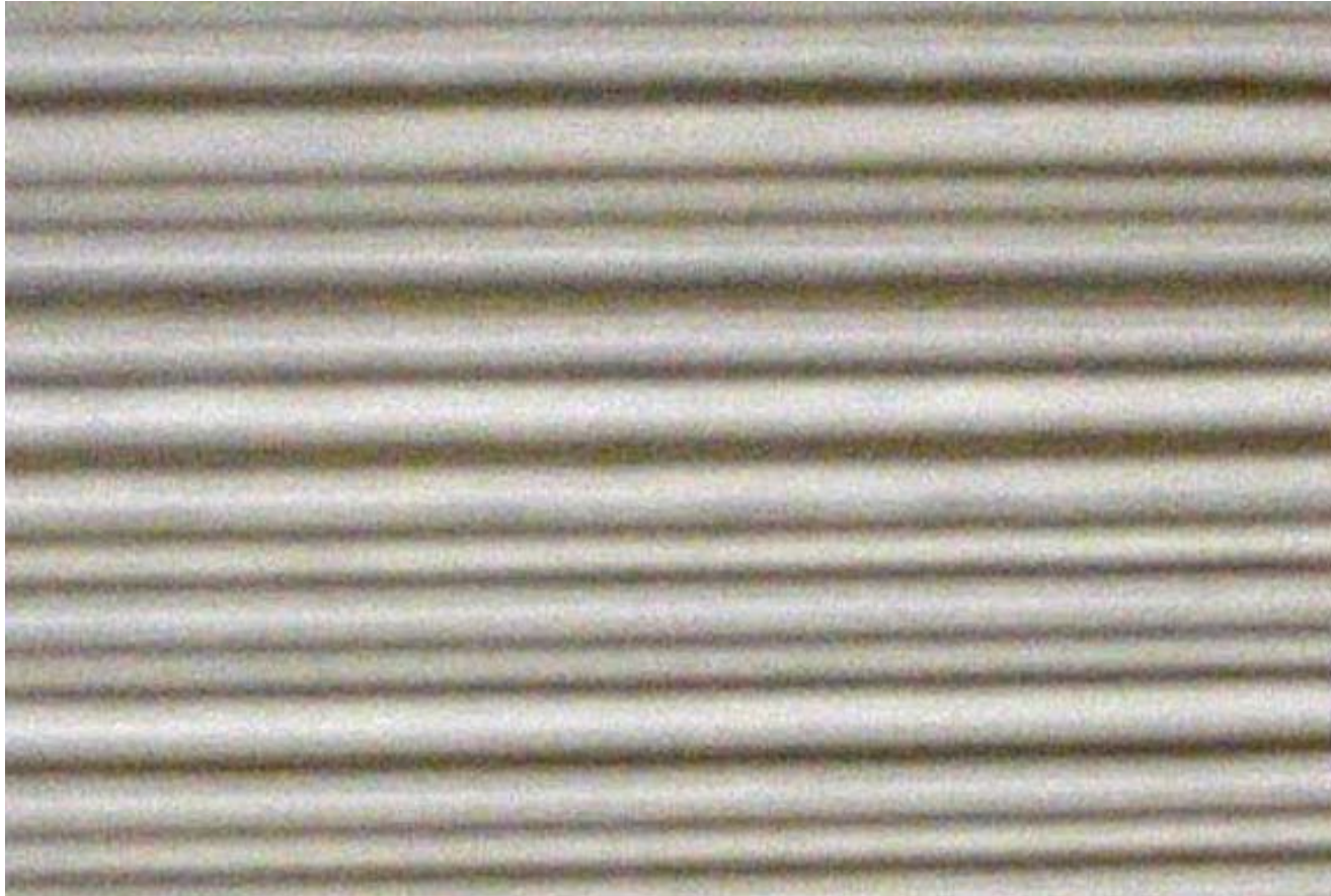
Figure 2b. Arrangement of the coated microporous hollow fibers in rectangular cross flow test module
