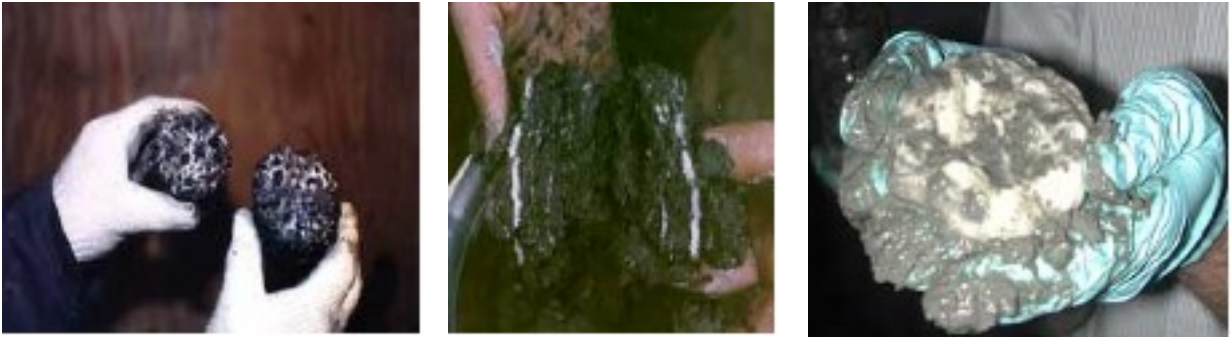
15 Figure 5.3. Photographs of methane hydrate as nodules, veins, and laminae in sediment. 16 Source: http://geology.usgs.gov/connections/mms/joint_projects/methane.htm .
