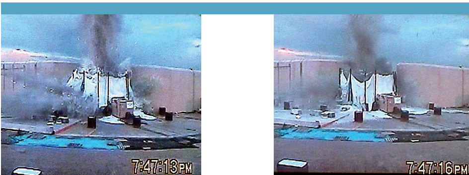
LEP MILESTONE: The latest hydrotest at DARHT, 3624, seen in this sequence of images, was accomplished with limited containment inside a shroud of fire-fighting-type foam intended to keep post-shot environmental cleanup to a minimum and greatly reduce fire danger. Future hydrotests at DARHT will be fully contained inside steel vessels.
