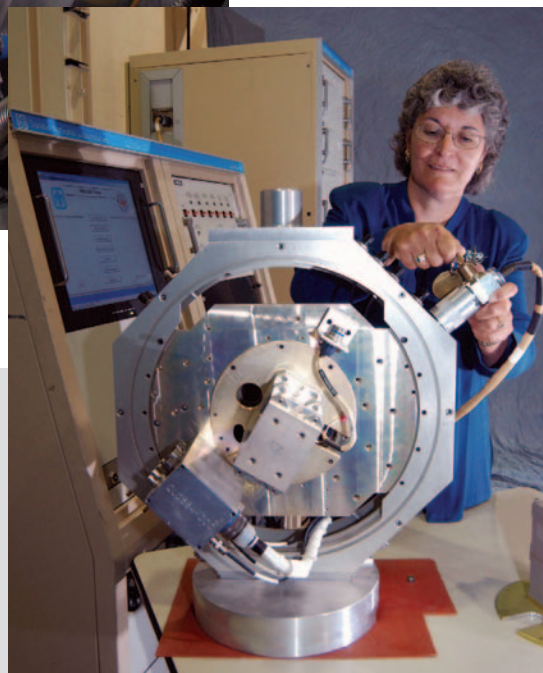
WEAPONS TESTING: Patricia Bonham examines Sandia's Command Disable System Tester, which is now in use at the Pantex Plant for weapons testing. Sandia engineers designed and built the tester.
