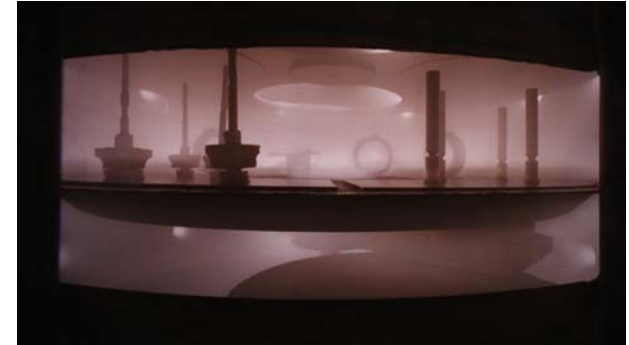
Near-Frictionless Carbon Film Being Applied to Engine Parts
