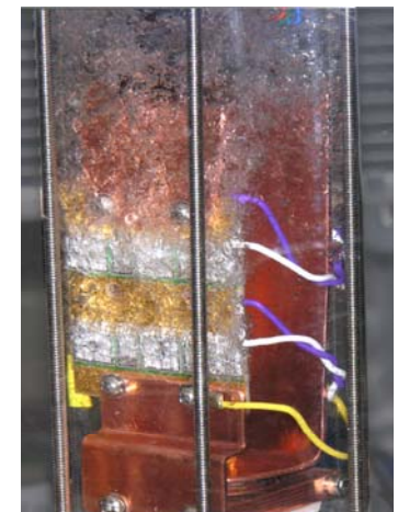
Silicon chip being directly cooled by liquid R134a coolant
