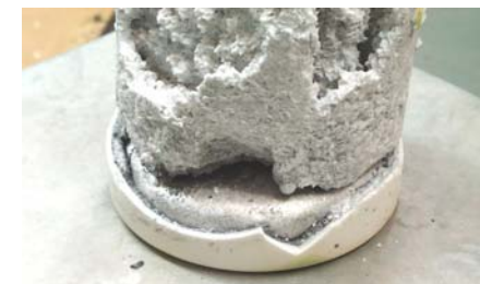
Commercial-grade aluminum produced from the Argonne inert-anode 100 Amp cell
