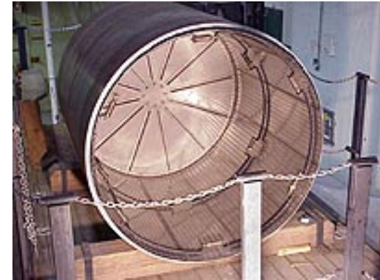
Multiport Dryer half-shell showing internal dryer insert.
