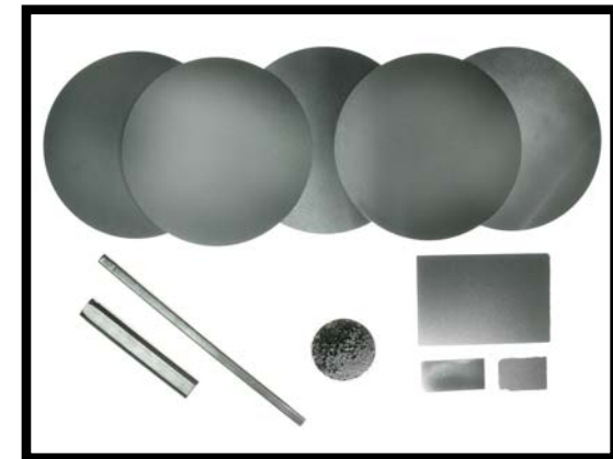
Low-Cost Titanium and Ti Alloy Plate, Bar, and Sheet Produced at ORNL
