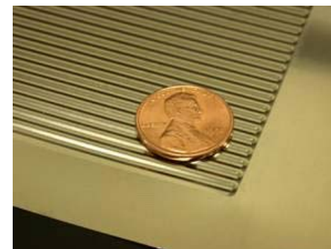
Stamped metallic bipolar plate (courtesy of GenCell Corp.)
