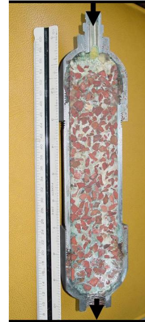
Laboratory simulation of sealing a lost circulation zone with a reactive plug
