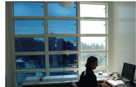
Windows darken when voltage is applied
