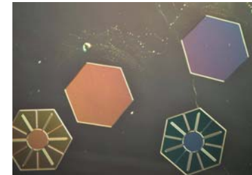
Create highly efficient thin/small cells ( 20 \mu\text{m} thick, 500 \mu\text{m} across).
