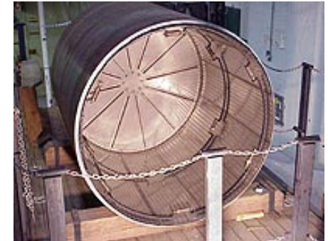
Multiport Dryer half-shell showing internal dryer insert.
