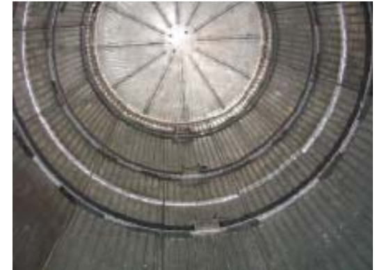
Multiport Dryer insert installed in a full-scale steam dryer
