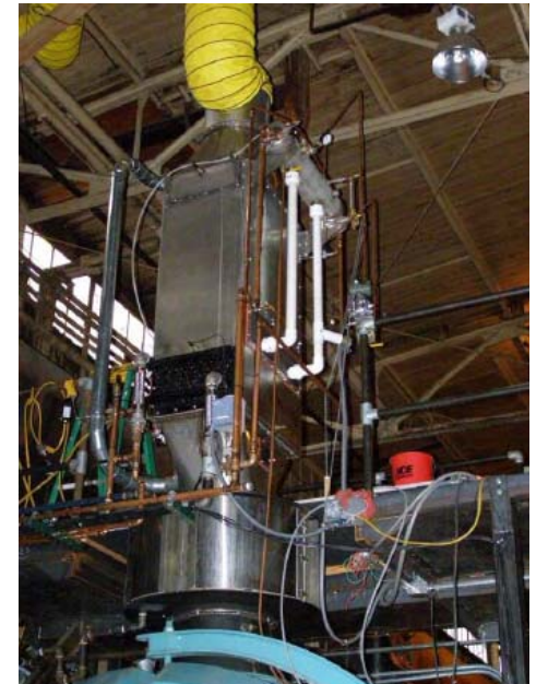
Full-size TMC module undergoing flue gas testing
