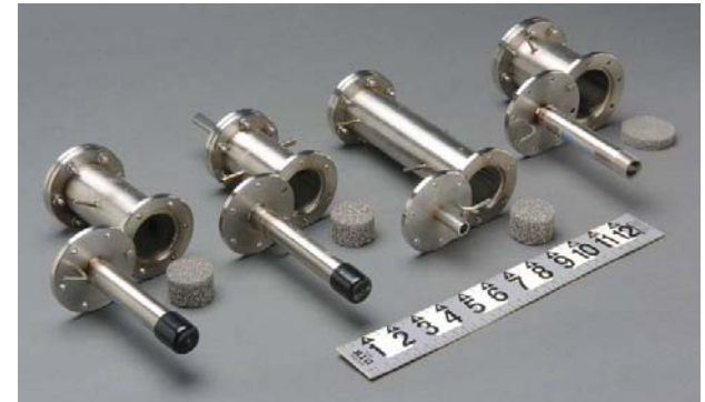
The reactor vessels above were developed for 1 to 2 kW e applications, and successfully tested in a breadboard configuration, validating the configurations and catalysts.
