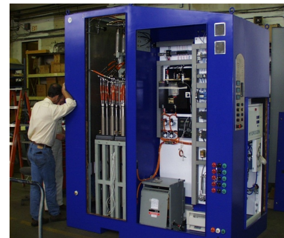
Typical Results – PV Driven Fueler with Integrated Storage and Dispenser
