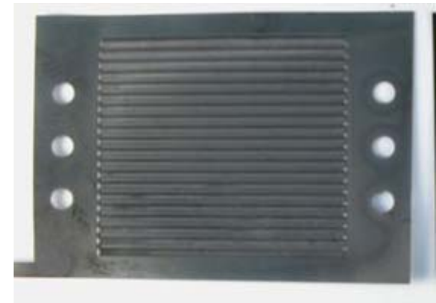
Stamped and nitrided 18 cm 2 active area bipolar plate (ORNL/GenCell Corp)
