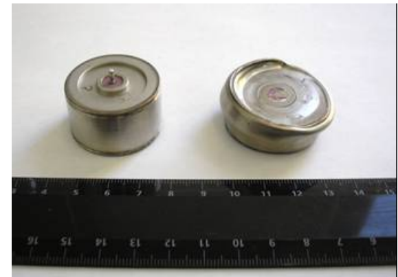
Intact battery (left) and one crushed at 250\text{ }^{\circ}\text{C} (right) with no thermal events or outgassing
