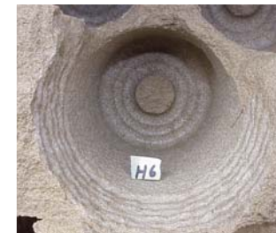
Well wall surface before (rough) and after damping (smooth)
