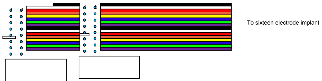
Figure 4. Ribbon cable used to connect two 8-channel bipolar modules to a 16-channel implant.
